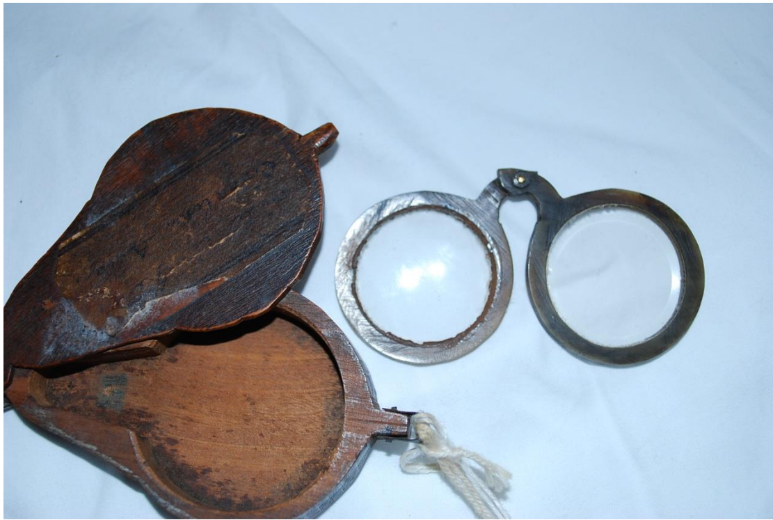
Horn pivot nosed spectacles with wooden case. One lens +2.0 diopter, other lens +5.0 c. 1760 (Hugh Orr Collection Sotheby's Olympia "Instruments of Science..." 28 th May 2003)
