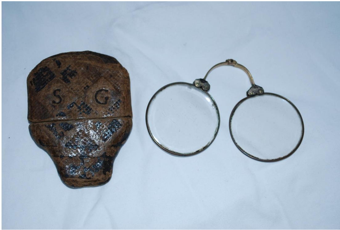
Pivot nose spectacles with faceted +3.0 diopter lenses and gilt copper rims and bridge with original paper banjo-style case c. 1740s (Hugh Orr Collection Sotheby's Olympia "Instruments of Science..." 28 th May 2003)
